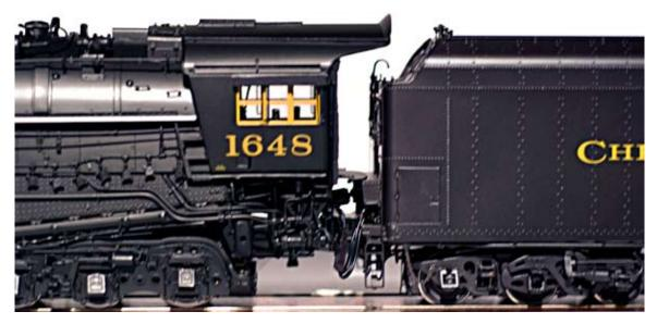
Shown above is the completed connection of the locomotive and tender, notice the position of the electrical connectors.
