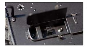
The photograph to the left shows the drawbar release hanging down under the operational buffer assembly. The prototypical double drawbar inserts into the two slots just above the release.
